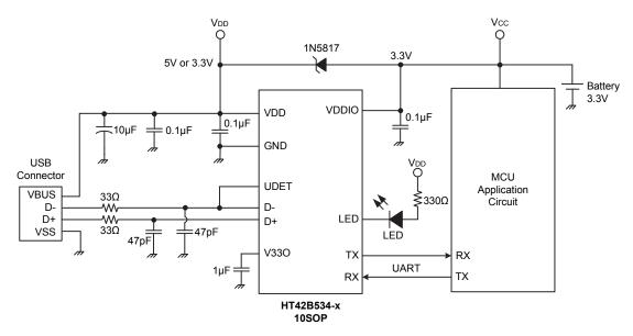
Note: 1. Design note: 10-SOP package only for two power application, the VCC power must be below VDD power. (The VCC power can be from the Li-battery).
