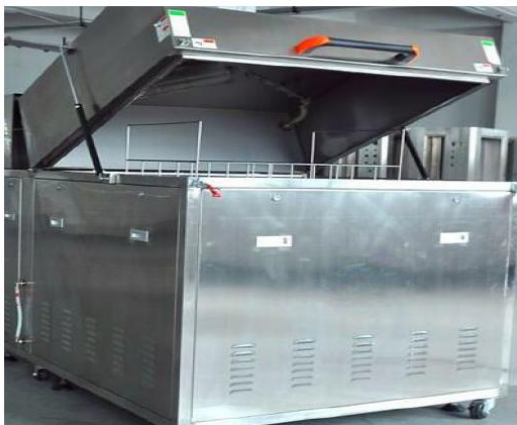
Pic.7 Tool spray cleaning
