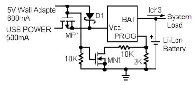
Fig.5:Combining Wall Adapter and USB Power
