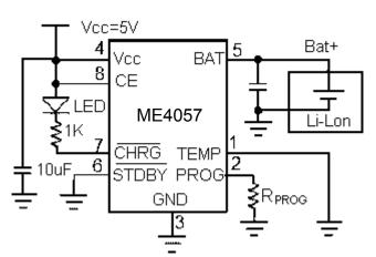
4. Suitable for the application which not need charge status indicator and battery's temperature detection.
