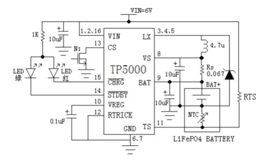
Figure 2 TP5000 is 3.6V 1.5A rechargeable lithium iron phosphate battery (150MA prefilled) Application Diagram
