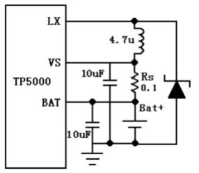
Figure 6 battery charging current setting
