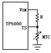
Figure 8 NTC connection diagram
