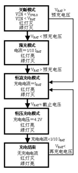
Figure 9 A typical lithium-ion battery charging cycle state diagram
