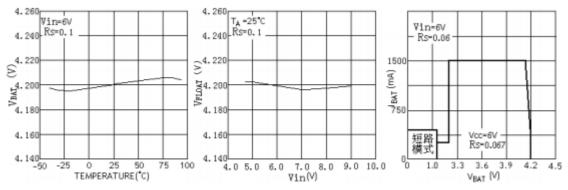
Cut-off voltage vs ambient temperature
