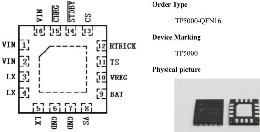
16-pin 4mm \* 4mmQFN16 Package Top View (Heat sink grounding unacceptable other potential)
