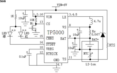
Figure 1 TP5000 is 1.5A 4.2V rechargeable lithium-ion battery (150MA prefilled) Application Diagram
