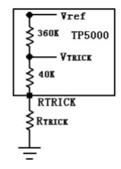
Figure 7 TRICK side view of the internal circuit diagram
