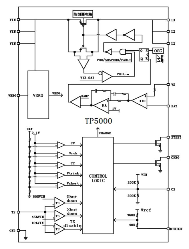
Figure 3 TP5000 Functional Block Diagram
