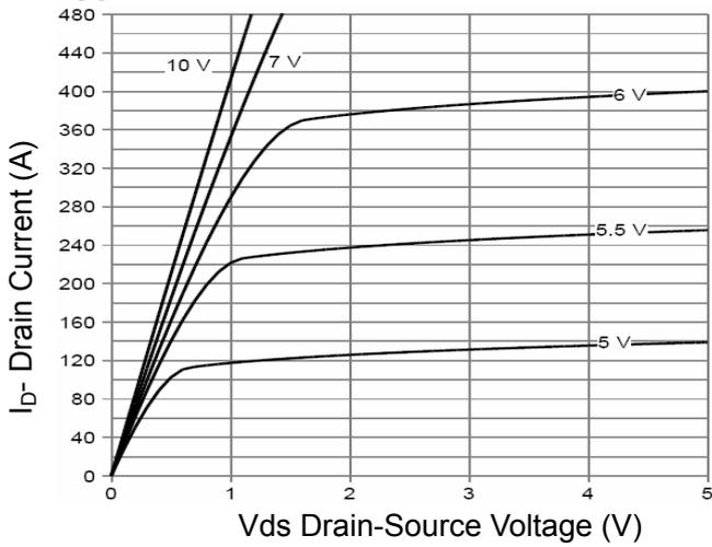
Figure 1 Output Characteristics
