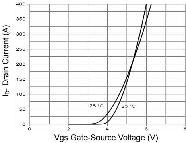
Figure 2 Transfer Characteristics
