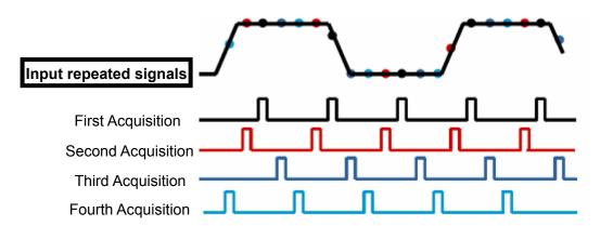
As shown above, acquire input signals (cycle repeatable) for more than once at a slow sample rate, arrange the sample points by the time they appear, then recover waveforms.
