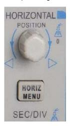
**1. HORIZONTAL POSITION Knob:** Used to control the trigger position against the screen center. Push this button to reset the trigger point back to the screen center.
