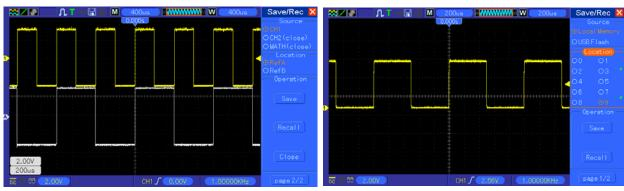
The white waveforms on the menu is the recalled RefA waveform
