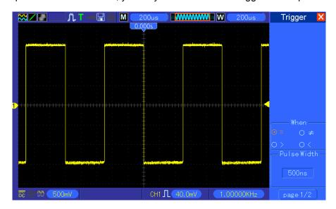
As shown in the above figure, you can get a stable waveform display if inputting a square wave at the frequency of 1KHz, with pulse width set to 500µs.
