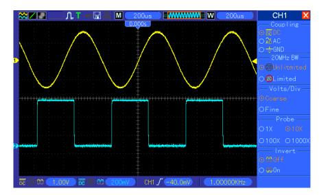
As illustrated in the above figure, input a 1KHz sine wave from CH1 and a 1KHz square wave from CH2.
