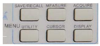
**SAVE/RECALL:** Displays the Save/Recall menu for setups and waveforms.
