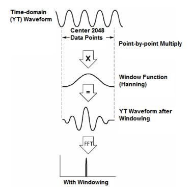
The Math FFT function has three FFT Window options. There is a trade-off between frequency resolution and amplitude accuracy for each type of window. You shall determine which one to choose according to the object you want to measure and the source signal characteristics.
