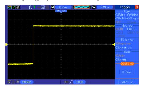
Note: The difference between the overtime and the delay triggers is that the overtime trigger can identify the pulse you need according to your set time and trigger on any point of the pulse. In the other word, the overtime trigger occurs based on pulse identification. It is similar to the > mode of the pulse width trigger, but not the same.
