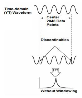
Applying a window to the YT waveform changes the waveform so that the start and stop values are close to each other, which reduces the discontinuities.
