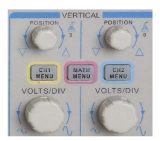
2. **Menu (CH1, CH2):** Display vertical menu options; turn on or off the display of channel waveforms.
