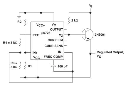
Figure 3. Negative-Voltage Regulator
