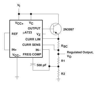
Figure 4. Positive-Voltage Regulator (External npn Pass Transistor)
