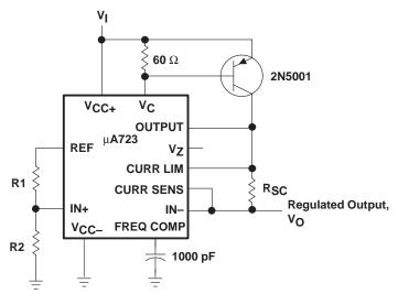
Figure 5. Positive-Voltage Regulator (External pnp Pass Transistor)
