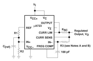
NOTES: A. R3 =  $\frac{R1 \times R2}{R1 + R2}$  for a minimum  $\alpha_{V_0}$  B. R3 can be eliminated for minimum component count. Use direct connection (i.e., R<sub>3</sub> = 0).
