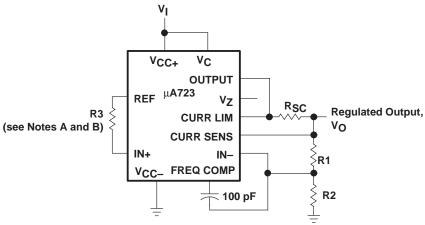
NOTES: A. R3 =  $\frac{R1 \times R2}{R1 + R2}$  for a minimum  $\alpha_{V_0}$ B. R3 can be eliminated for minimum component count. Use direct connection (i.e., R<sub>3</sub> = 0).
