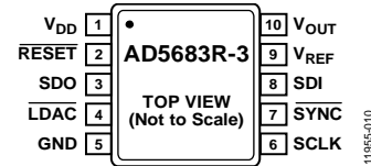
Figure 10. Pin Configuration, 10-Lead MSOP, SDO Option
