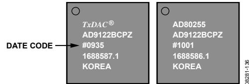
Figure 36. Revision 1 Silicon, AD9122BCPZ Marking
