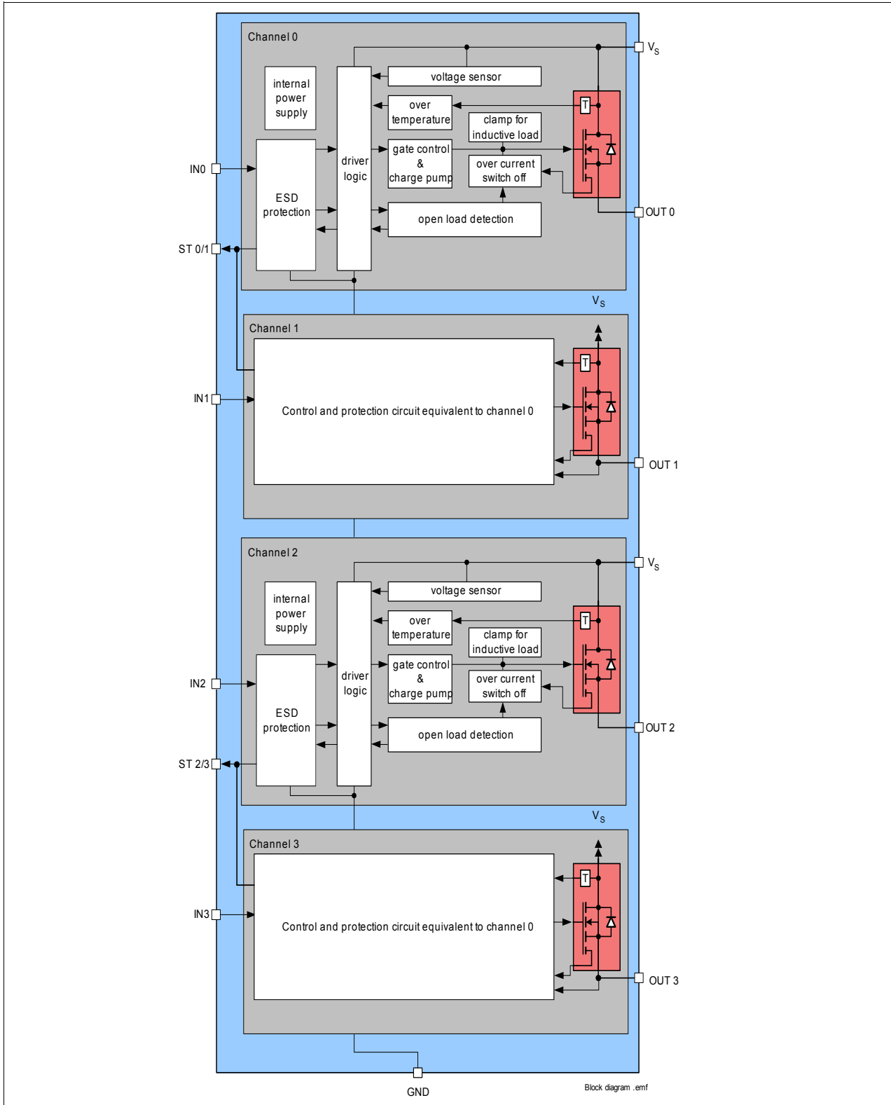
Figure 1 Block diagram for the BTS4130QGA
