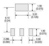
Dimensions mm MIN / mm MAX (inches MIN / inches MAX)
