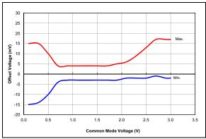
**FIGURE 36-83:** Comparator Offset, NP Mode (CxSP = 1), VDD = 3.0V, Typical Measured Values at 25°C.
