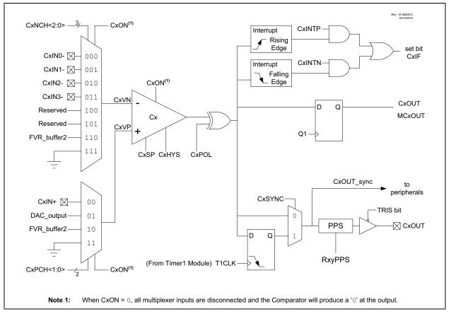
FIGURE 19-2: COMPARATOR MODULE SIMPLIFIED BLOCK DIAGRAM
