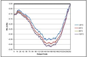
**FIGURE 36-93:** Typical DAC INL Error, VDD = 3.0V, VREF = External 3V.
