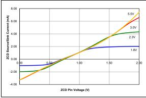
**FIGURE 36-103:** ZCD Pin Current over ZCD Pin Voltage, Typical Measured Values from -40°C to 125°C.
