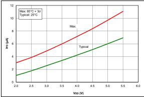
FIGURE 36-32: IPD, Timer1 Oscillator, Fosc = 32 kHz, PIC16F1614/8 Only.
