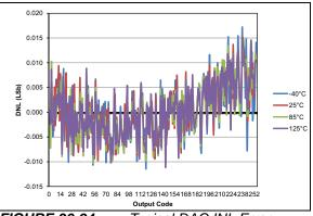
**FIGURE 36-94:** Typical DAC INL Error, VDD = 5.0V, VREF = External 5V, PIC16F1614/8 Only.
