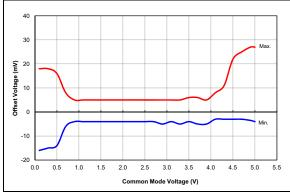
**FIGURE 36-87:** Comparator Offset, NP Mode (CxSP = 1), VDD = 5.5V, Typical Measured Values From -40°C to 125°C, PIC16F1614/8 Only.
