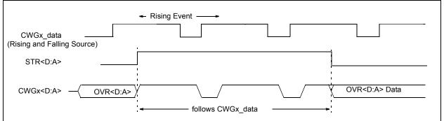
FIGURE 28-11: EXAMPLE OF STEERING EVENT AT BEGINNING OF INSTRUCTION (MODE<2:0> = 001)
