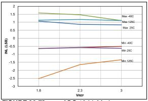
**FIGURE 36-72:** ADC 10-bit Mode, Single-Ended INL, VDD = 3.0V,  $TAD = 1 \mu S$ .
