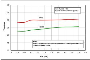
FIGURE 36-64: FVR Stabilization Period, PIC16LF1614/8 Only.
