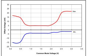
**FIGURE 36-84:** Comparator Offset, NP Mode (CxSP = 1), VDD = 3.0V, Typical Measured Values From -40°C to 125°C.
