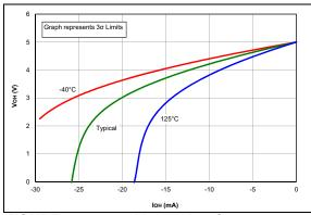
**FIGURE 36-37:** VOH vs. IOH Over Temperature, VDD = 5.0V, PIC16F1614/8 Only.
