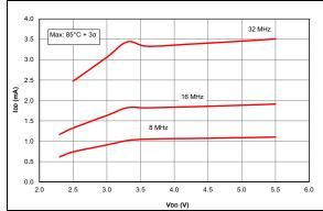
FIGURE 36-20: IDD Maximum, HFINTOSC Mode, PIC16F1614/8 Only.
