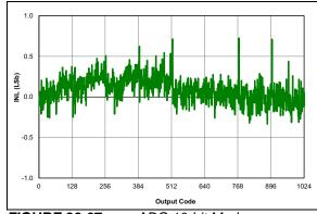
**FIGURE 36-67:** ADC 10-bit Mode, Single-Ended INL, VDD = 3.0V, TAD =  $1 \mu$ S,  $25^{\circ}$ C.
