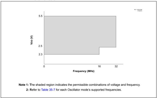
FIGURE 35-2: VOLTAGE FREQUENCY GRAPH, -40°C  $\leq$  Ta  $\leq$  +125°C, PIC16LF1614/8 ONLY
