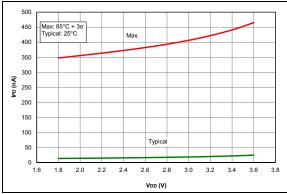
FIGURE 36-33: IPD, ADC Non-Converting, PIC16LF1614/8 Only.
