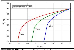
FIGURE 36-41: VOH vs. IOH Over Temperature, VDD = 3.0V.
