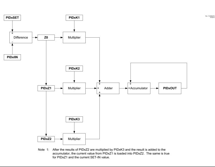
Within the controller, the input is subtracted from a preprogrammed set point to get an error value. This error value, along with the previous two error values (if any), are multiplied by user-input coefficients and the results of these multiplications are added together to make up the output. If the MODE<2:0> bits of the PIDxCON register = 101, the PID output is equal to the current output added to any previous outputs.
