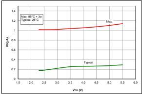
FIGURE 36-34: IPD, ADC Non-Converting, PIC16F1614/8 Only.
