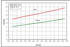
FIGURE 36-28: IPD, Brown-Out Reset (BOR), BORV = 1, PIC16F1614/8 Only.
