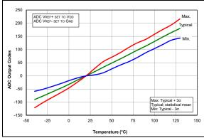
**FIGURE 36-79:** Temp. Indicator Slope Normalized to 20°C, Low Range, VDD = 1.8V, PIC16LF1614/8 Only.
