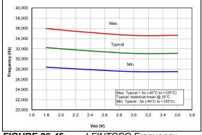
FIGURE 36-45: LFINTOSC Frequency, PIC16LF1614/8 Only.
