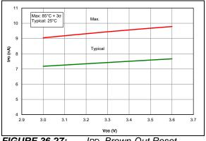
*FIGURE 36-27: IPD, Brown-Out Reset* (BOR), BORV = 1, PIC16LF1614/8 Only.
