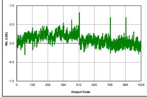
**FIGURE 36-68:** ADC 10-bit Mode, Single-Ended INL, VDD = 3.0V, TAD =  $4 \mu$ S,  $25^{\circ}$ C.
