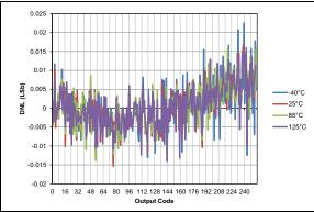
**FIGURE 36-92:** Typical DAC DNL Error, VDD = 3.0V, VREF = External 3V.
