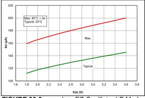
FIGURE 36-3: IDD, EC Oscillator LP Mode, Fosc = 500 kHz, PIC16LF1614/8 Only.
