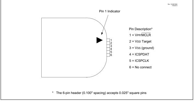
For additional interface recommendations, refer to your specific device programmer manual prior to PCB design.
