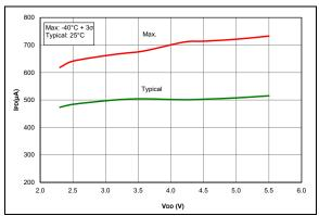
**FIGURE 36-36:** IPD, Comparator, NP Mode (CxSP = 1), PIC16F1614/8 Only.
