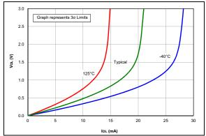
**FIGURE 36-42:** Vol vs. Iol Over Temperature, VDD = 3.0V.
