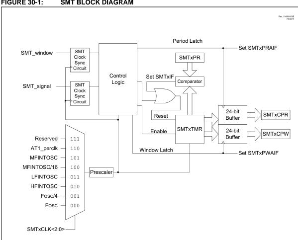
FIGURE 30-1: SMT BLOCK DIAGRAM
