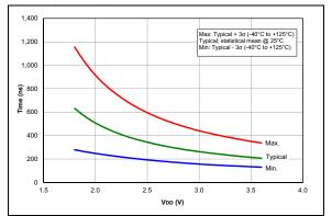
**FIGURE 36-90:** Comparator Output Filter Delay Time Over Temp., NP Mode (CxSP = 1), Typical Measured Values, PIC16LF1614/8 Only.
