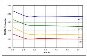
**FIGURE 36-101:** ZCD Pin Voltage, Typical Measured Values.
