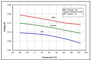
**FIGURE 36-53:** Brown-Out Reset Voltage, High Trip Point (BORV = 0).
