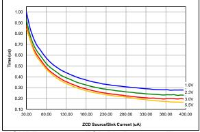
**FIGURE 36-104:** ZCD Pin Response Timer over Current, Typical Measured Values from -40°C to 125°C.
