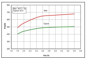
**FIGURE 36-35:** IPD, Comparator, NP Mode (CxSP = 1), PIC16LF1614/8 Only.
