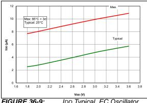
FIGURE 36-9: IDD Typical, EC Oscillator HP Mode, PIC16LF1614/8 Only.
