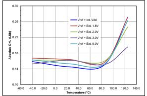
FIGURE 36-99: Absolute Value of DAC DNL Error, VDD = 5.0V, VREF = VDD, PIC16F1614/8 Only.
