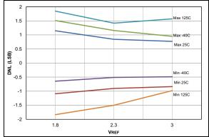
**FIGURE 36-71:** ADC 10-bit Mode, Single-Ended DNL, VDD = 3.0V,  $TAD = 1 \mu S$ .
