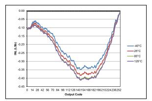
FIGURE 36-95: Typical DAC INL Error, VDD = 5.0V, VREF = External 5V, PIC16F1614/8 Only.
