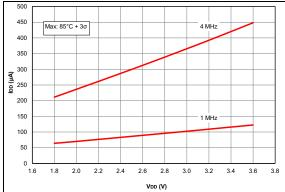
FIGURE 36-14: IDD, LFINTOSC Mode, Fosc = 31 kHz, PIC16F1614/8 Only.
