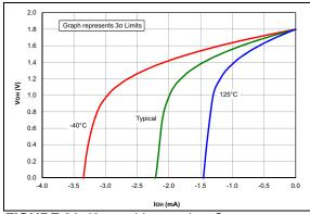
FIGURE 36-43: Voн vs. Ioн Over Temperature, VDD = 1.8V, PIC16LF1614/8 Only.
