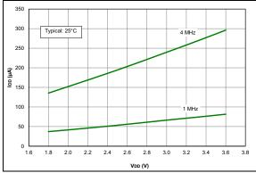
FIGURE 36-13: IDD, LFINTOSC Mode, Fosc = 31 kHz, PIC16LF1614/8 Only.
