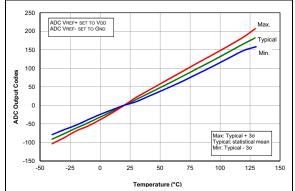
**FIGURE 36-81:** Temp. Indicator Slope Normalized to 20°C, High Range, VDD = 3.6V, PIC16LF1614/8 Only.
