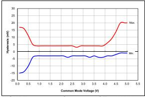
**FIGURE 36-86:** Comparator Offset, NP Mode (CxSP = 1), VDD = 5.0V, Typical Measured Values at 25°C, PIC16F1614/8 Only.
