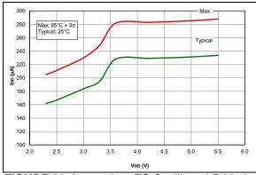
FIGURE 36-4: IDD, EC Oscillator LP Mode, Fosc = 500 kHz, PIC16F1614/8 Only.
