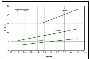
FIGURE 36-17: IDD Typical, HFINTOSC Mode, PIC16LF1614/8 Only.
