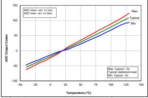
**FIGURE 36-80:** Temp. Indicator Slope Normalized to  $20^{\circ}$ C, Low Range, VDD = 3.0V, PIC16LF1614/8 Only.
