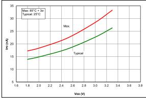
FIGURE 36-25: IPD, Fixed Voltage Reference (FVR), PIC16LF1614/8 Only.
