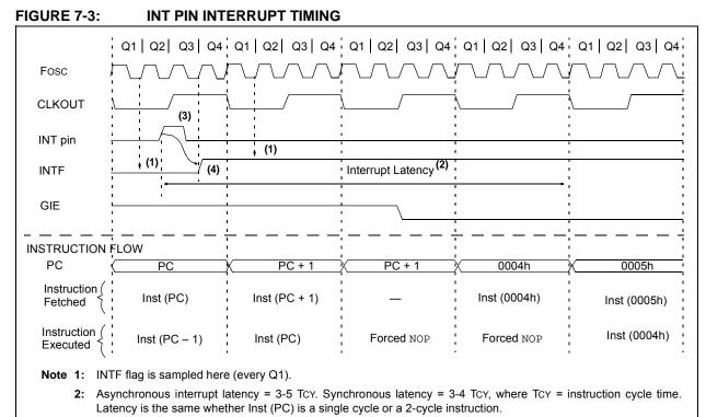
3: For minimum width of INT pulse, refer to AC specifications in Section35.0 "Electrical Specifications".
