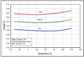
FIGURE 36-59: POR Release Voltage.
