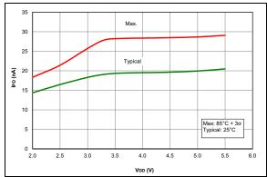
FIGURE 36-26: IPD, Fixed Voltage Reference (FVR), PIC16F1614/8 Only.
