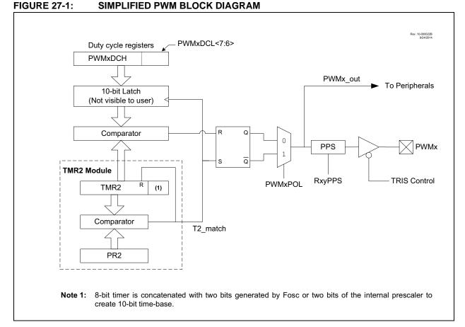
Figure 27-1 shows a simplified block diagram of PWM operation.
