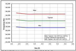
FIGURE 36-46: LFINTOSC Frequency, PIC16F1614/8 Only.
