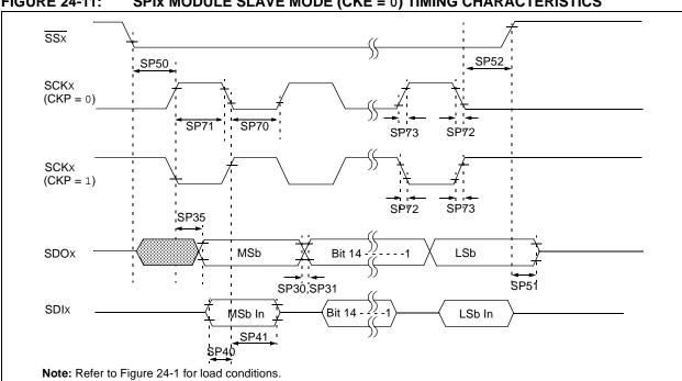
FIGURE 24-11: SPIX MODULE SLAVE MODE (CKE = 0) TIMING CHARACTERISTICS
