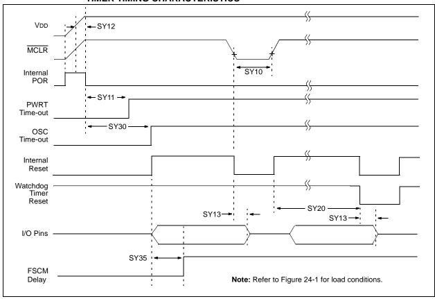
TABLE 24-21: RESET, WATCHDOG TIMER, OSCILLATOR START-UP TIMER, POWER-UP TIMER TIMING REQUIREMENTS
