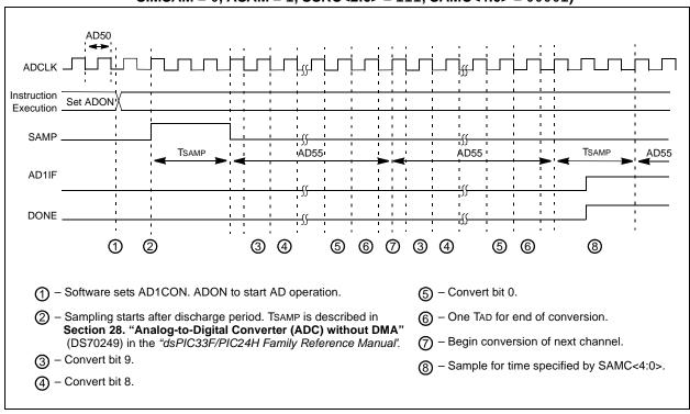
TABLE 24-39: ADC CONVERSION (10-BIT MODE) TIMING REQUIREMENTS
