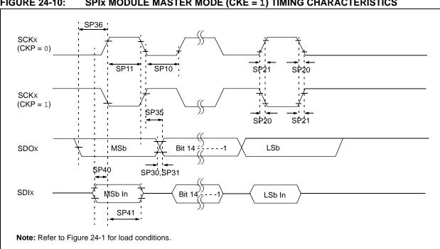
FIGURE 24-10: SPIX MODULE MASTER MODE (CKE = 1) TIMING CHARACTERISTICS
