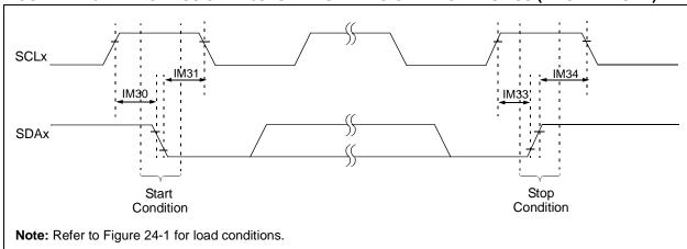
FIGURE 24-14: I2Cx BUS DATA TIMING CHARACTERISTICS (MASTER MODE)
