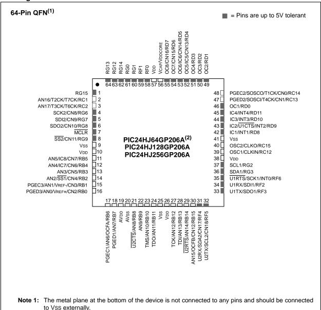
2: The PIC24HJ64GP206A device does not have the SCL2 and SDA2 pins.
