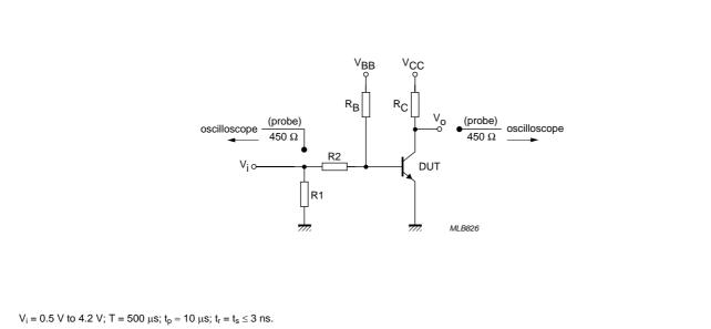
R1 = 56  $\Omega$ ; R2 = 1 k $\Omega$ ; R<sub>B</sub> = 1 k $\Omega$ ; R<sub>C</sub> = 270  $\Omega$ .
