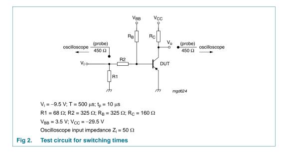
40 V, 600 mA PNP switching transistor
