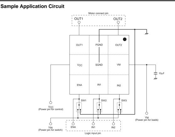
\* Connect a kickback absorbing capacitor as close as possible to the IC. Characteristics deterioration of the IC or damage may result if an instantaneous voltage surge exceeding the maximum rated value is applied to the VM line due to coil kickback or other causes.
