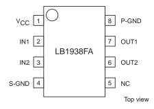
S-GND: GND for the control system P-GND: GND for the power system
