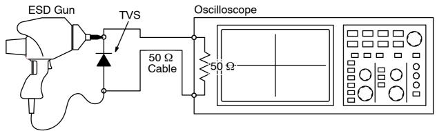
Figure 4. Diagram of ESD Test Setup
