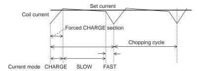
The IC switches to SLOW DECAY after Blanking section, and then switches to FAST DECAY mode for the last about 1µs.
