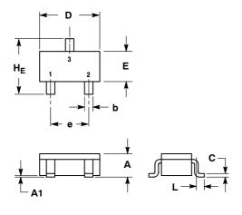
NOTES: 1. DIMENSIONING AND TOLERANCING PER ANSI Y14.5M, 1982. 2. CONTROLLING DIMENSION: MILLIMETER.
