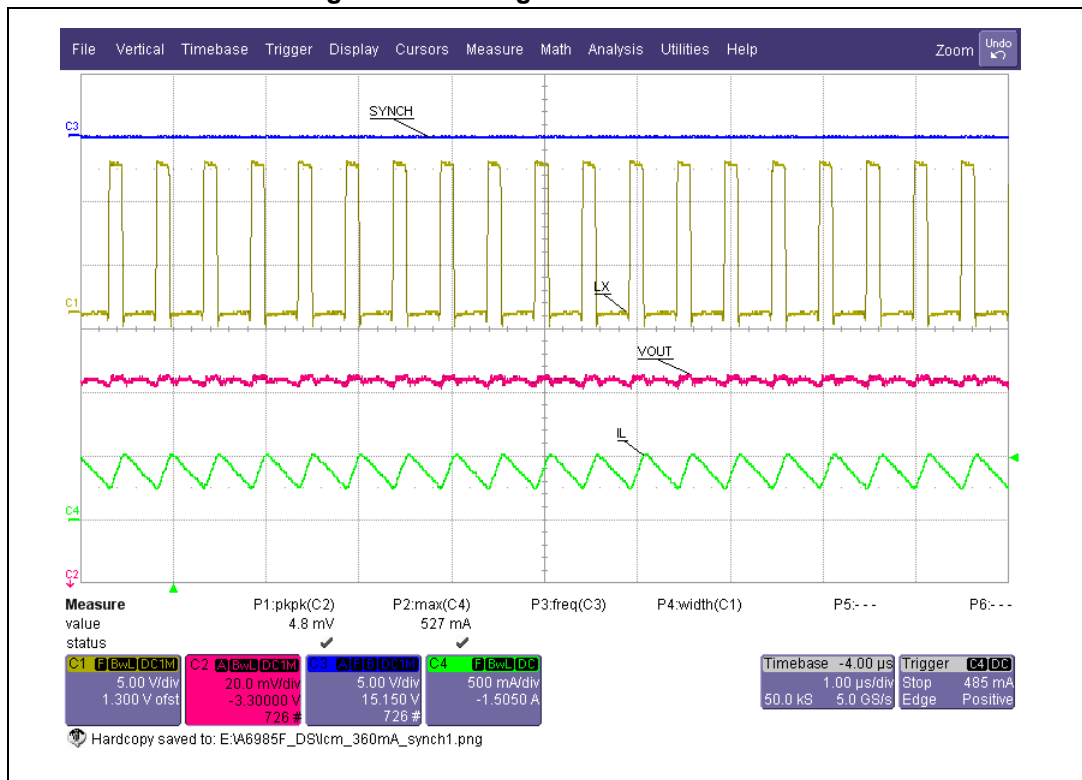
Figure 20. The regulator works in CCM
