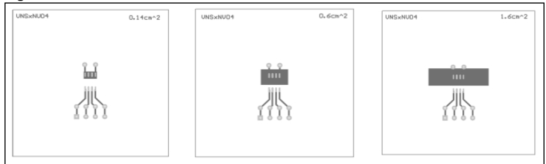
Figure 37. SO-8 PC board (1)
